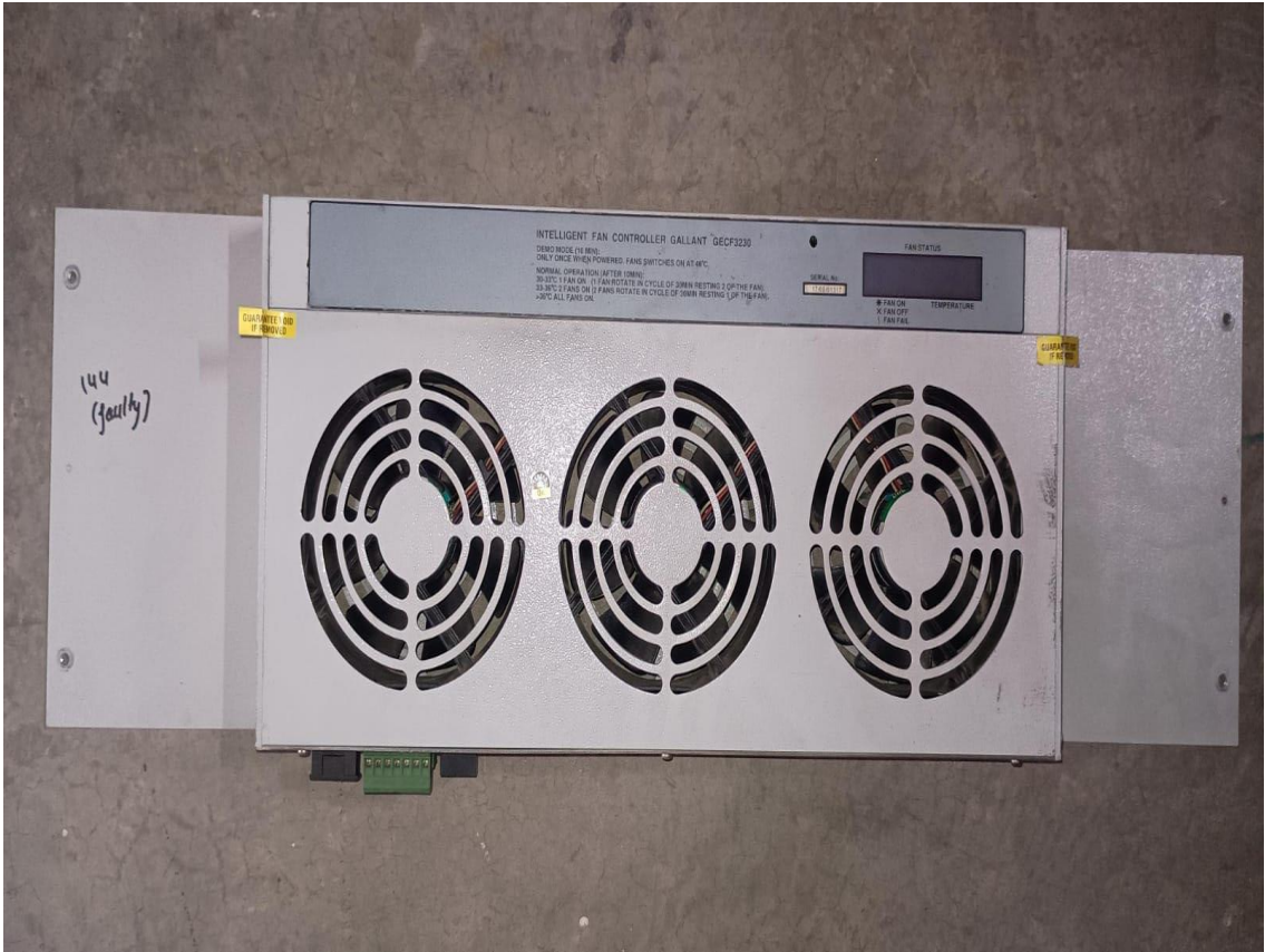
Fig. 4 Intelligent Temperature Monitor and Controller Unit
