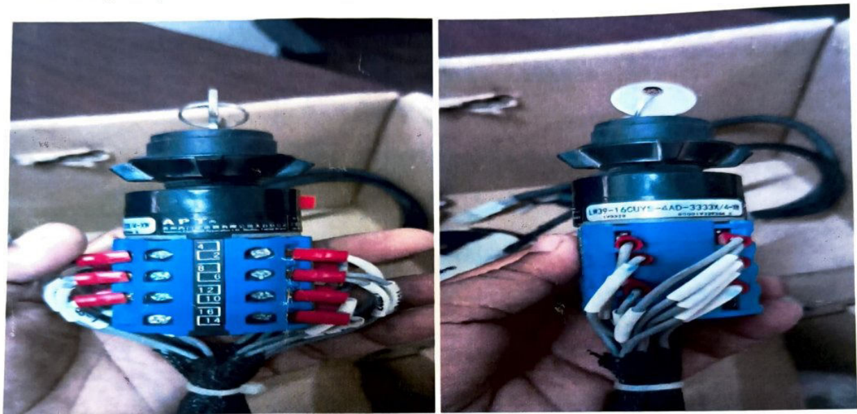
LCB ASD (Rotary Selection switch 4 position with key) (part no. LW39-16CUYS-4AD-3333X/4-XW)
