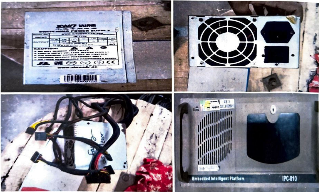
SMPS for CPU (I/P 110V DC, O/P +3.3V, +5V, +12V, -12V, +5VSB), 350 watt
